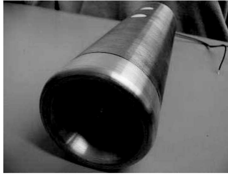
Figure 7: New design of gerdien tube.
