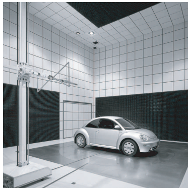
Figure 1: Semi anechoic chamber lined ferrite tiles. (Ferrite tiles are installed back of the white interior finishing panel. Pyramidal ferrite absorbers are installed back of the black color rea).
