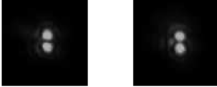
Figure 3: Two different equilibrium states of a 2.3\ \mu\text{m} doublet. The main difference is the interference pattern. On the first picture, droplets are emitting in phase opposition, we see a dark fringe on the symmetry axis. On the second one, they are emitting in phase, bright dots can be seen on the symmetry axis. It suggests that the difference of separation distance between droplets increased. We estimated the increasing to be of the order of half a wavelength in accordance with the interference pattern.
