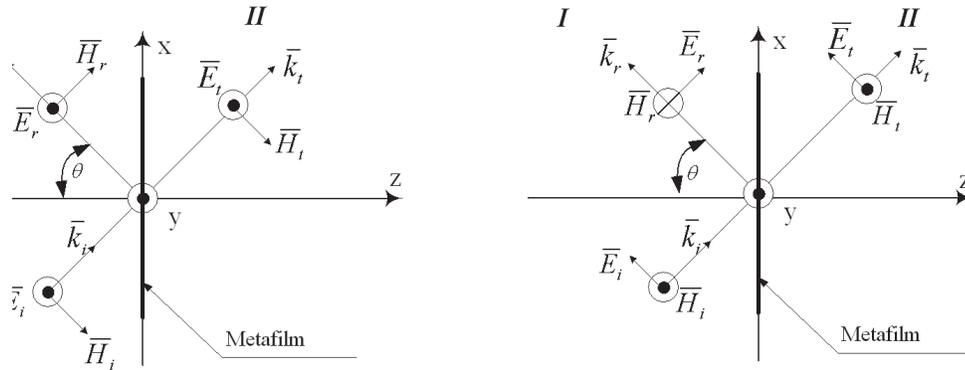
Figure 2: TE and TM polarized plane waves.
