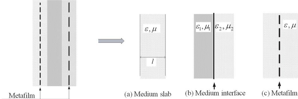
Figure 1: Decomposition of multilayered MF.
