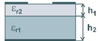
Figure 1: Cross-section of the CBSL with a stacked substrate.
