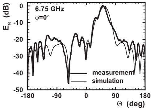
Figure 13: Radiation pattern of the antenna from Fig. 12 at 6.75 GHz.
