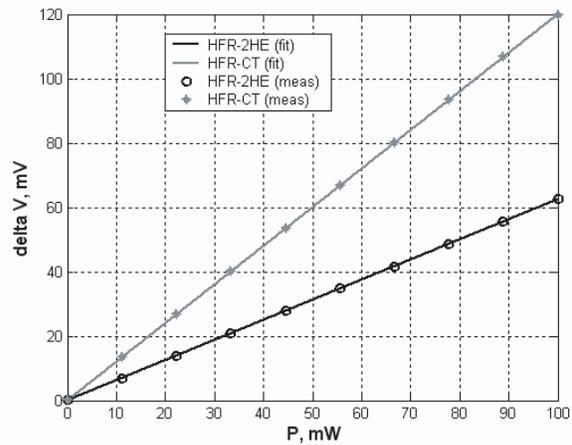
Figure 3: Linear volt-watt characteristics for transducers.
