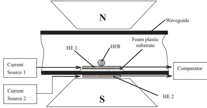
Figure 1: Schematic of the transducer based on the HFR and two Hall-elements.
