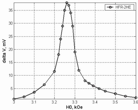
Figure 2: Resonance dependence of the converted voltage (HFR-2 Hall elements).
