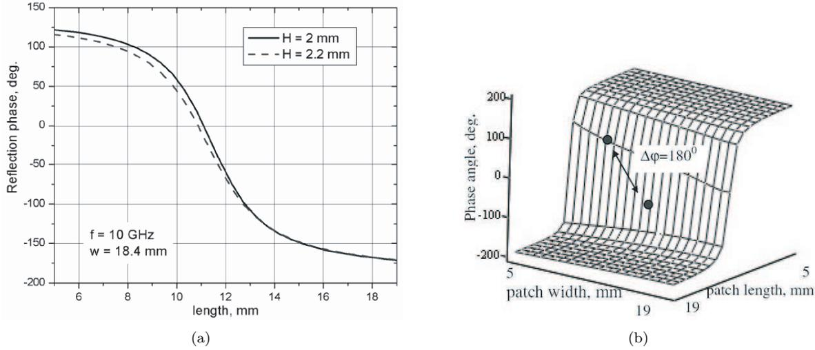
Figure 2: Results of calculation of phase angle depending on patch dimensions (a) Phase angle versus length of patch (different thickness of the substrate  $H$ ), (b) Surface plot of phase angle in dependence on both dimensions of patch. Frequency 10 GHz, thickness of substrate  $H = 2$  mm, dielectric permittivity 1.06,  $L = 21$  mm, range of patch sizes 5–19 mm.
