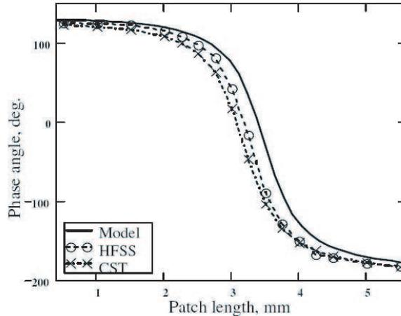
Figure 4: Comparison of simulation by presented model and by using microwave simulation packages.  $H = 0.787$  mm,  $\epsilon_r = 2.22$ ,  $L = 6$  mm, range of patch sizes from 0.6 to 5.6 mm,  $f = 25$  GHz.
