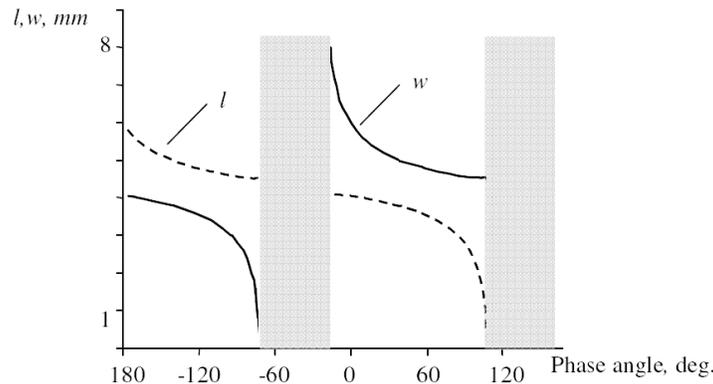
Figure 3: Dependence of phase angle on patch dimensions.
