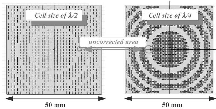
Figure 6: 50 mm diameter reflectors with uncorrected zones.
