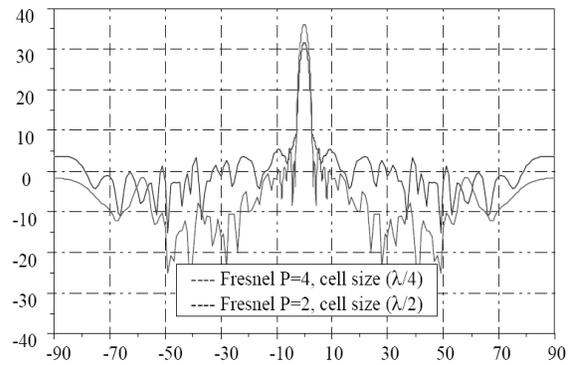
Figure 5: Simulated radiation pattern of Fresnel reflectors with  $D = 100$  mm.
