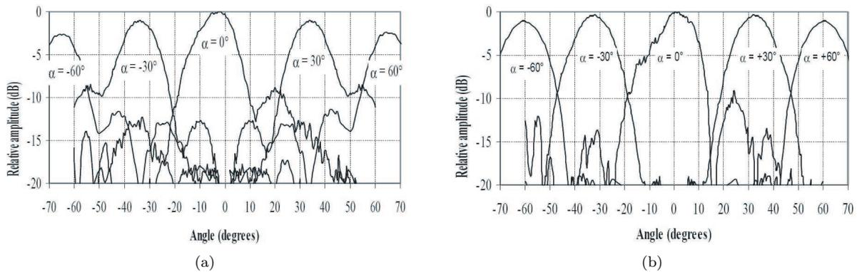
Figure 3: (a)  $D = 1(\lambda/2)$  cell size, (b)  $\lambda/4$  cell size.
