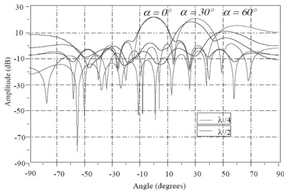
Figure 4: Simulated radiation pattern of the 15 mm reflectarray with different cell sizes.
