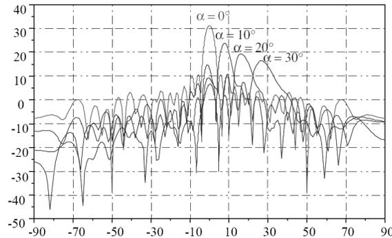
Figure 7: Simulated radiation pattern showing the limitation of cell sizes reduction.
