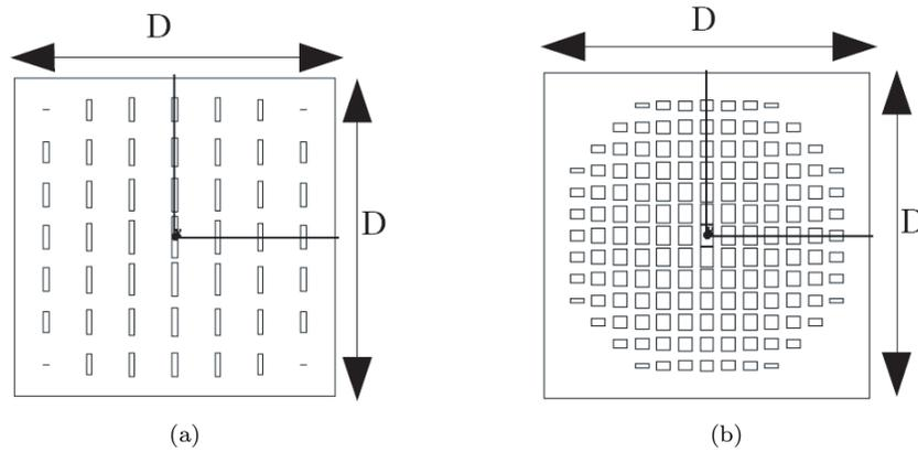
Figure 1: (a)  $\lambda/2$  cell, (b)  $\lambda/4$  cell.
