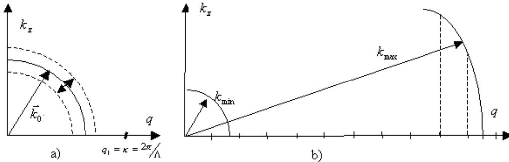
Figure 2: The range of wave numbers change for narrowband -(a) and UWB -(b) signal.
