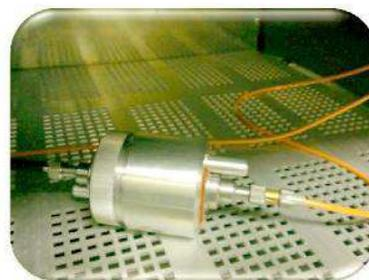
Figure 4: The fiber optic device with the capsule for fixing the tested specimen inside of the heating-cooling chamber.
