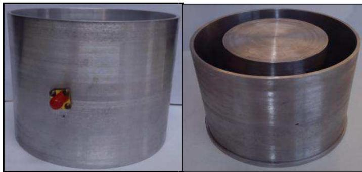
Figure 5: Fabricated input cavity.
