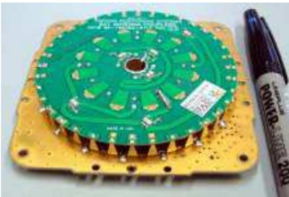
Figure 7: Concentric L1/L2 antenna.
