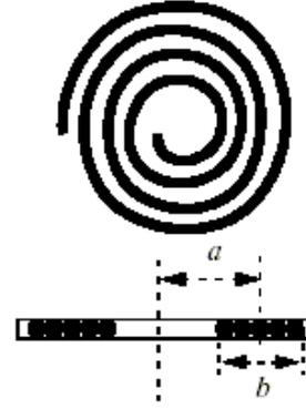
Figure 3: Spiral plate coil parameters.
