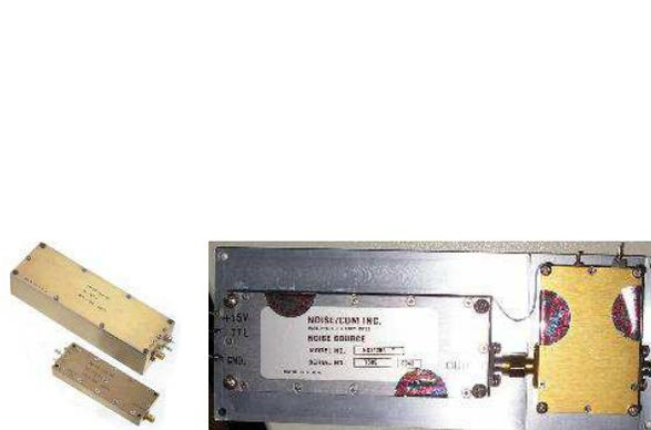
Figure 2: The applied noise generator and power amplifier. The image shows the tested noise generator, whose output power is 0 dBm in the frequency range of between 100 kHz and 10 GHz.
