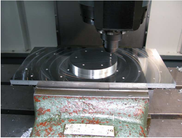
Figure 4: The milling of the surface areas of the main load-bearing part of a telescope.
