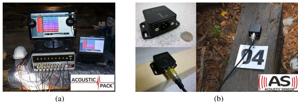
Figure 7: The realized acoustic diagnostic system. (a) Terrain workplace. (b) Detail of the acoustic sensor.
