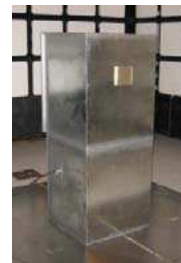
Figure 3: Ventilation panel installed in the real shielding casing.
