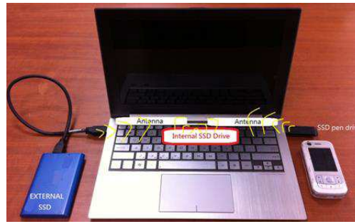
Figure 1: Scenario of WiFi tethering with mobile phone placed aside of SSD.
