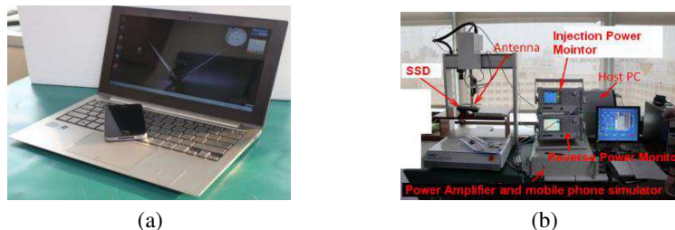
Figure 6: (a) Test condition for mobile phone placed beside the SSD. (b) The PNS setup for EMS test using mobile phone simulator.
