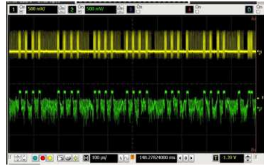
Figure 3: Oscillogram for USB 2.0 interface during transmission of information data sequence consisting of logic zeroes. Yellow colour — directly from interface transmission line. Green colour — signal at output of amplitude detector of eavesdropping receiver tuned to frequency f = 240 MHz.
