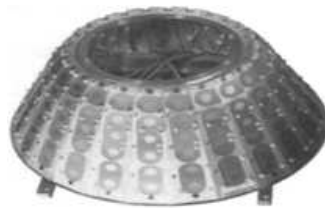
Figure 1: Conformal array antenna for missile-borne.
