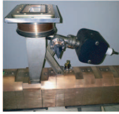
Figure 9: Side view of the tuned window on the LINAC.
