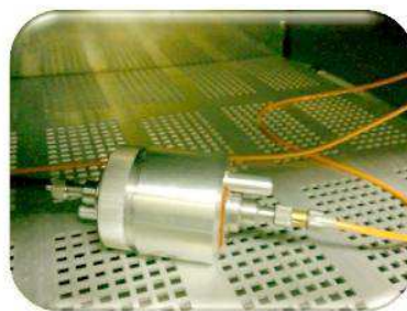
Figure 4: The fiber optic device with the capsule for fixing the tested specimen inside of the heating-cooling chamber.
