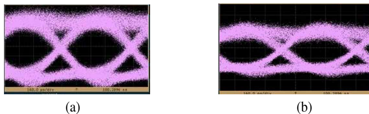
Figure 4: Electrical eye diagrams in (a) back-to-back and (b) 12.5 km transmission scenarios.
