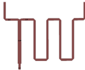
Figure 10: The last power divider schematic.
