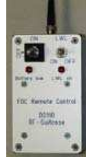
Figure 4: Remote control switch generator Diehl DS 110.
