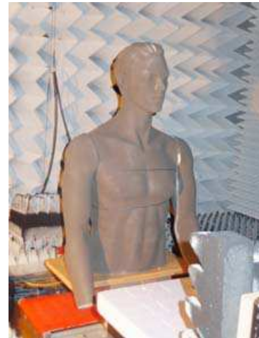
Figure 2: Metal-coated mannequin on a moving platform used in our radar measurement.
