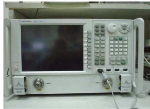
Figure 6: A agilent N5245A PNA-X network analyzer.
