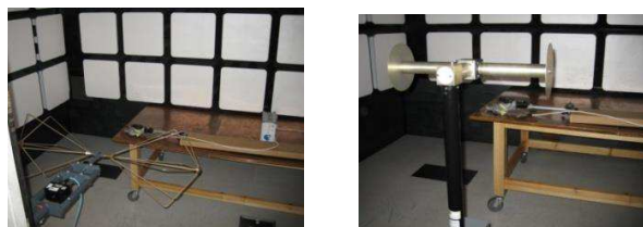
Figure 4: Laboratory stand for radiated disturbances measurement.
