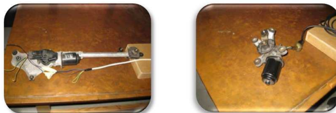
Figure 1: Motors of windscreen wipers of Subaru Forester II and I.
