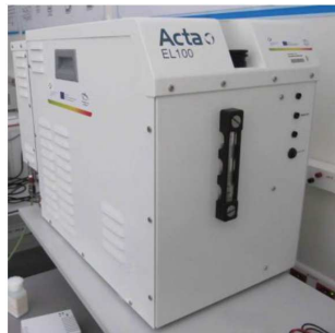
Figure 2: The hydrogen generator ACTA EL100c + dryer.
