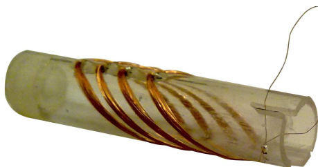
Figure 3: Prototype induction coil with 100 turns on cylindrical acrylic tube.
