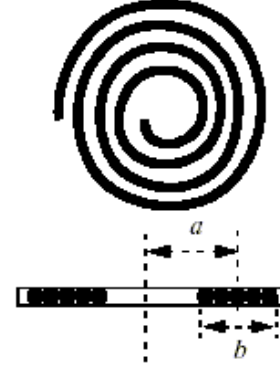
Figure 3: Spiral plate coil parameters.
