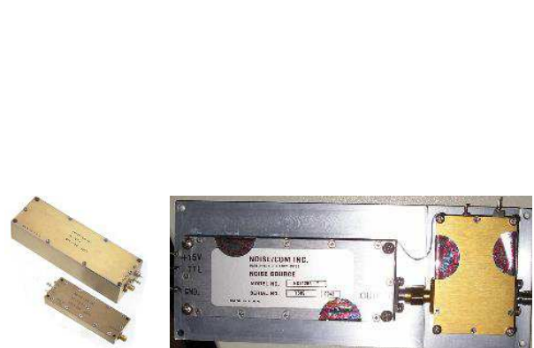
Figure 2: The applied noise generator and power amplifier. The image shows the tested noise generator, whose output power is 0 dBm in the frequency range of between 100 kHz and 10 GHz.
