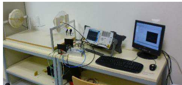
Figure 4: The arrangement of the noise spectroscopy station (free room).
