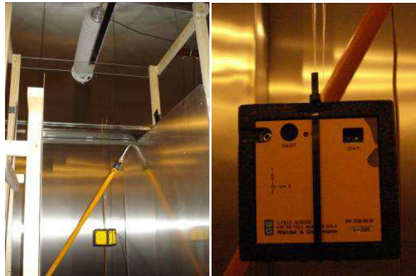
Figure 2: Method 2 — sensor fixed using plastic clamp and three fishing lines.
