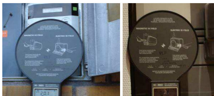
Figure 1: Examples of electric field measurements of houses with smart meter.
