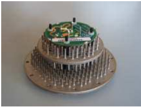
Figure 3: Dual band patch antenna with comb substrates.
