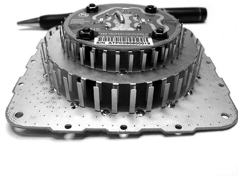
Figure 4: Dual band patch antenna with capacitive frame.
