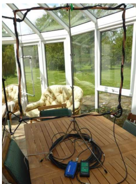
Figure 3: 70 cm sided square copper loop foldable loop-monopole with MiniVNApro and battery operated XGA3 DDS signal generator below.
