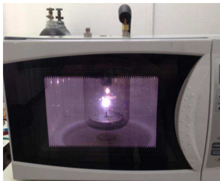
Figure 4: Photograph of plasma generation in ethanol vapor.
