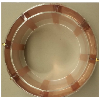
Figure 4: Eight-channels MTL RF coil prototype.
