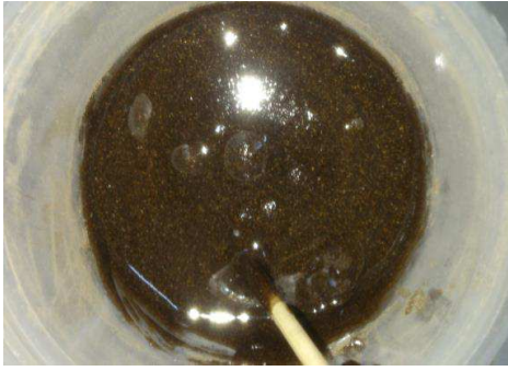
Figure 1: RHCNTs after stir with polyester and MEKP.
