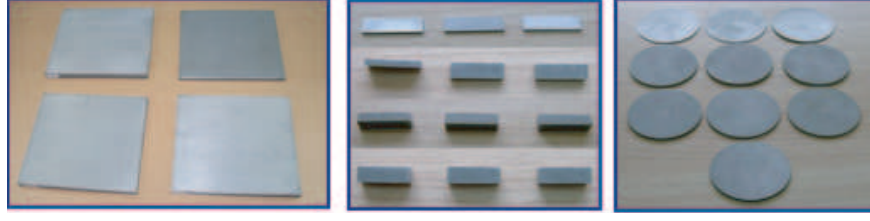
Figure 3: The scaled simulated composite material samples of the seawater.
