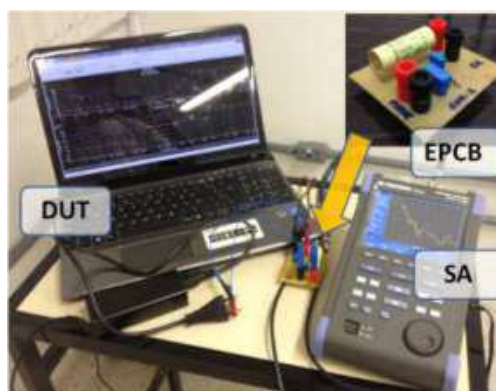
Figure 2: Conducted emission test setup using an EPCB.
