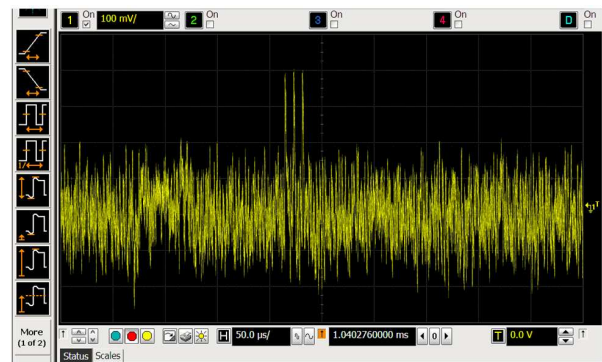
Figure 6: Oscillogram for laser printer connected to PC and printing test pattern b). The signal received by antenna for f = 220 MHz from VIDEO output of FSET22 receiver.
