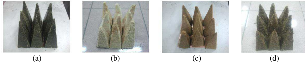
Figure 1: 3 \times 3 array pyramidal microwave absorber. (a) Rice husk-rubber tire dust. (b) Sugarcane bagasse. (c) Rice husk. (d) Banana leaf.
